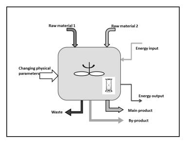
Fig. 1. Batch process scheme.
